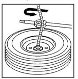
The wheel wrench has a hook that allows you to pull the hoist cable towards you to assist in reaching the spare tire.
